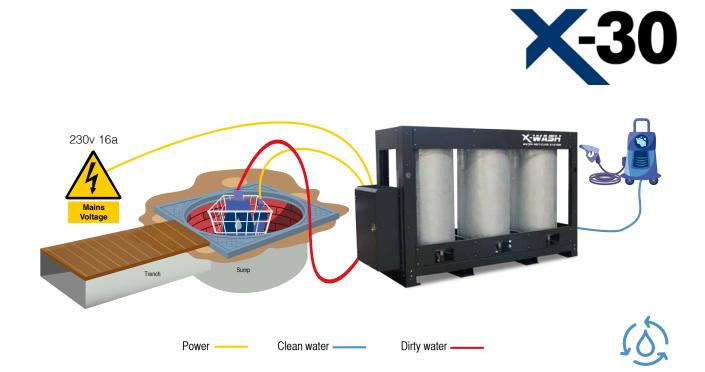
The dirty water from the Interceptor collection tank is typically made up by a range of contaminants such as sand and mud in suspension, aggregates and residues of hydrocarbons. This requires a variet of filters to remove these pollutants.
