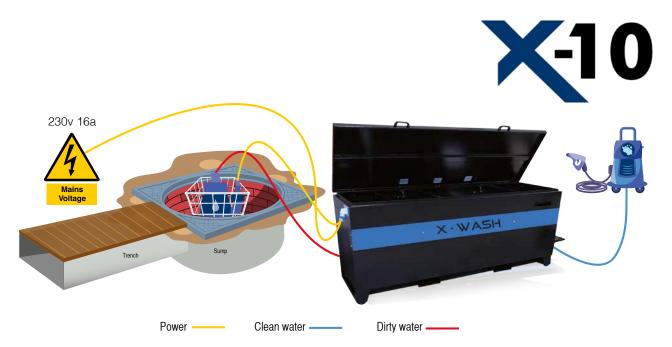
The dirty water from the Interceptor collection tank is typically made up by a range of contaminants such as sand and mud in suspension, aggregates and residues of hydrocarbons. This requires a variety of filters to remove these pollutants.
