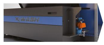
Water is pumped into this tank from the X-Wash collection tank. This tank contains more filters.
