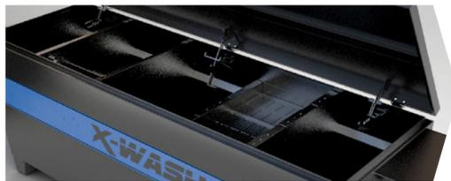
The filtration tank contains four sections with filters to remove oil and fuel deposits.
